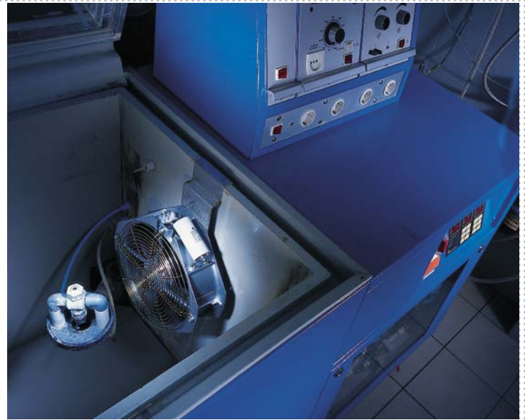
FIGURE 6: Fans often have to withstand harsh ambient conditions and therefore pass through various test stations beforehand, such as the salt spray test at ebm-papst.
