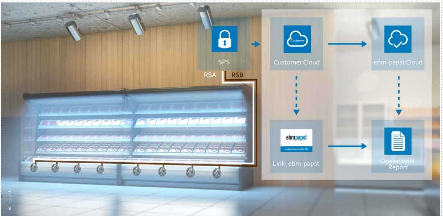
FIGURE 5: The intelligent EC motors in the fans in refrigerated display cases also supply data for cloud analysis.
