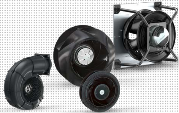
FIGURE 4: Centrifugal fans perform particularly well against high back pressures. They are available with forward or backward-curved blades and in a scroll housing or as freewheel fans as appropriate. They are typically implemented in central ventilation units.
