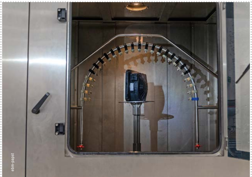
FIGURE 3: In the IP test chamber, electronics and fans are subjected to standardized degree of protection tests in accordance with the IP code against moisture ingress. The tests at ebm-papst are supplemented by long-term climate tests to represent a load over a longer period of time.
