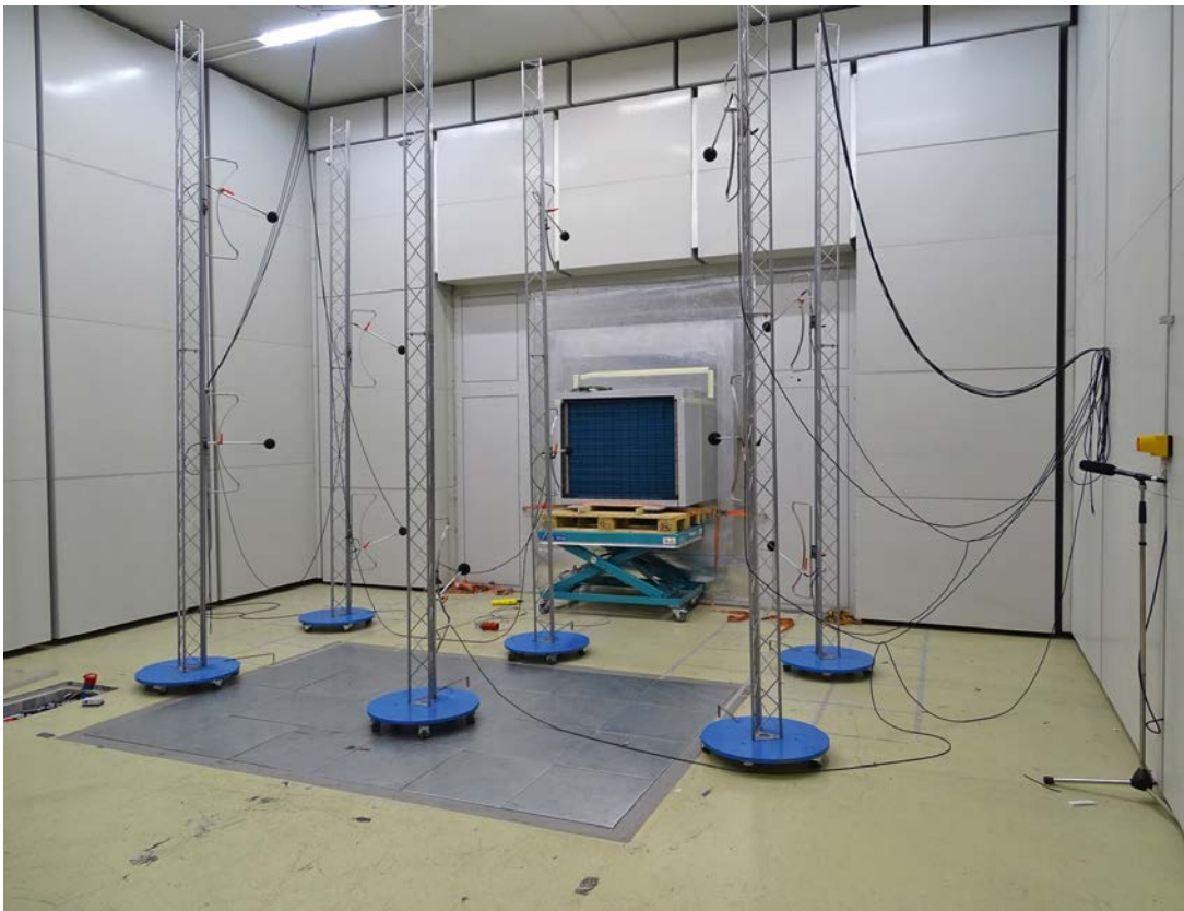
FIGURE 4: In this measuring device, noises are recorded via a variety of microphones and then played to the test subjects for evaluation.
