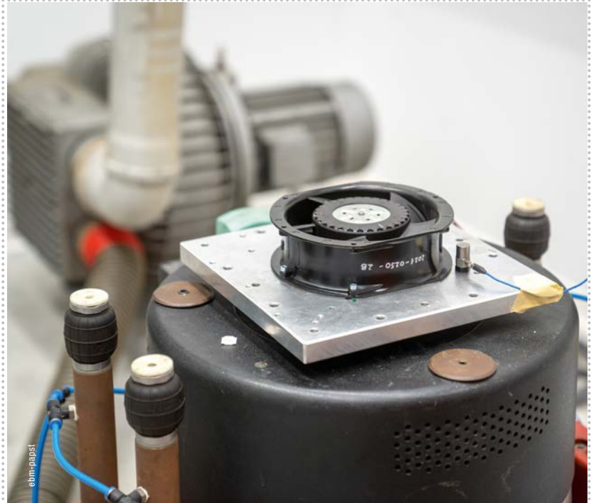
FIGURE 10 + 11: The shock and vibration test bay simulates the loads caused by transport by train, truck, ship or aircraft. The test bench carries out sustained vibrations of varying strengths and individual shock pulses.
