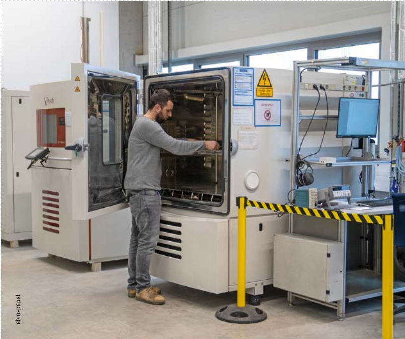
FIGURE 4: In several climatic chambers, a temperature increase or drop can be generated within a very short time.
