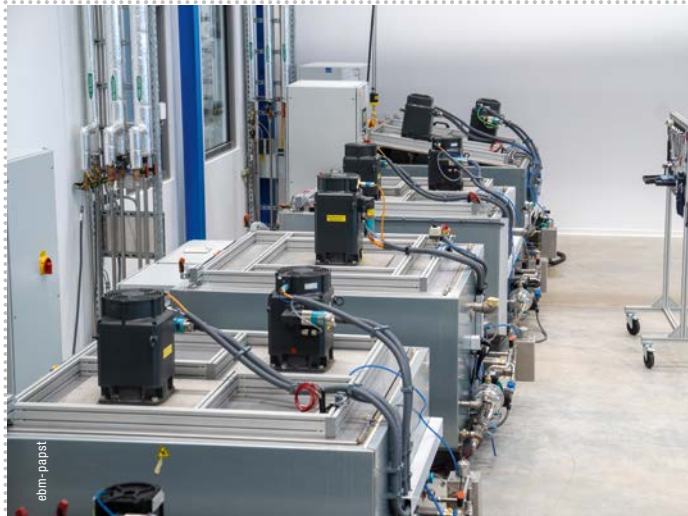
FIGURE 7: The wheel strength of smaller or larger fans is checked at various stations.
