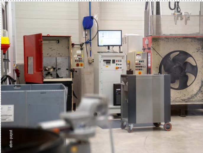
FIGURE 8: In plastic impellers, the 'growth of the flowing material' is analyzed via the centrifugal load. The maximum permissible speed is exceeded many times over.
