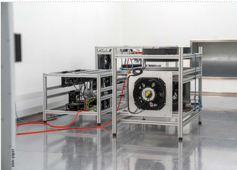
FIGURE 5: In addition to standardized test procedures, ebm-papst has developed its own 'combined load tests', which the test objects are subjected to throughout the entire product development process.
