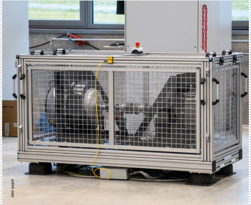
FIGURE 2: The FanDrive DV280 also has to pass tests. It is the largest EC external rotor motor ever built by ebm-papst and reaches a torque of 180 Nm at a power output of 24 kW.
