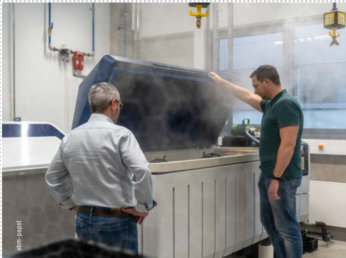
FIGURE 6: The quality of the coatings and materials is investigated in the salt spray test chamber.
