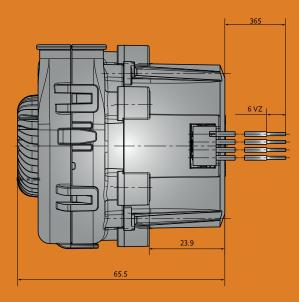
For plastic-cutting screws Ø 2.5 mm max. screw-in depth 6 mm
