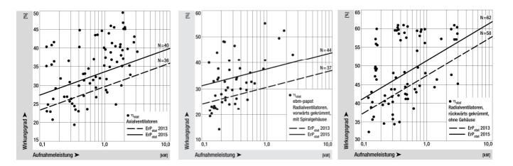
Efficiency Input capacity Axial fans Centrifugal fans, forward curved, with scroll housing Centrifugal fans, forward curved, without housing
