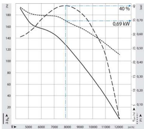
For the HyBlade® axial fan illustrated with a drive input power of 0.69 kW at best operating point, the formula states that an efficiency of at least 28.65% must be achieved by 2013 and at least 32.65% by 2015, based on the static pressure increase. The curve indicates 40% efficiency, which is already substantially higher than the minimum requirement for 2015. This fan thus already satisfies the future specifications.
